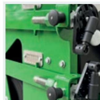
PRECISION: Spindles to adjust installation height and compaction.
