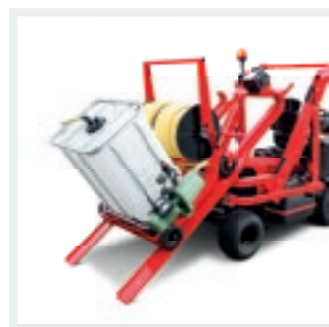
INDIVIDUAL: Ramp with winch for trolley with 300 litre intermediate tank, water pump and 2x 75 mtr. hoses.
