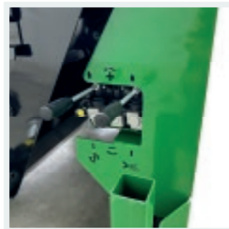
PROTECTED: Steering elements integrated in the chassis.
