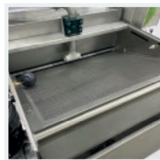
Belt filter with tear-proof filter fleece (120 µm) including collecting container with float switch
