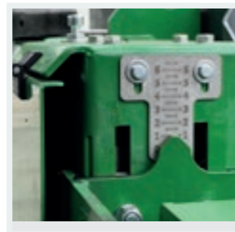
PRECISION: Electric spindles on the screed bar with sensors and scale.
