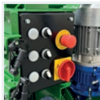
SIMPLE: Central control panel including all operating functions.
