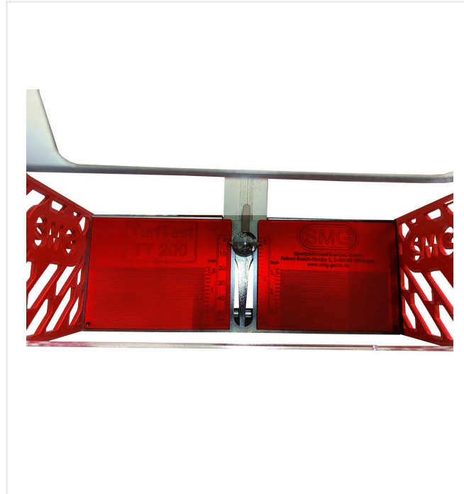
measuring free pile height
